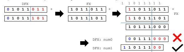
• Addition of two *num*1 numbers. Addition results in overflow (we need 9 bits to represent the result). Here, the result in format  $8_{-3}^{-2}$  has to include an overflow flag. We can recover from this if we include a carry out ( $c_n$ ) bit in the circuitry.
