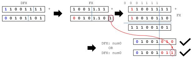
• Subtraction of two *num*1 numbers. The operation does not result in overflow, *num*0 suffices to represent the final result in the 8\_3\_2 format.
